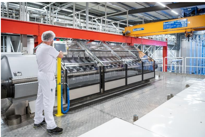
In the butter press, the freshly processed organic cocoa mass is carefully pressed to separate the liquid cocoa butter from the solid press cake from which cocoa powder is made. (Photo: © PRONATEC AG)
